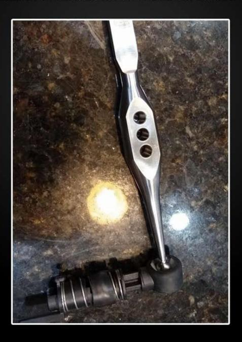
STEP 12: NOW YOU WILL NEED TO INSTALL THE SHIFT LEVER BY PLACING THE 2 SPACERS ON THE INSIDE OF THE BEARINGS. YOU CAN USE SOME GREASE TO HOLD THEM IN PLACE. SLIDE THE SHIFT LEVER IN AND PUSH PIN THROUGH TO DESIRED THROW POSITION. TIGHTEN THE 8MM FLANGE NUT AND USE LOCKTITE TO PREVENT IT FROM COMING LOOSE. SEE PICS.
