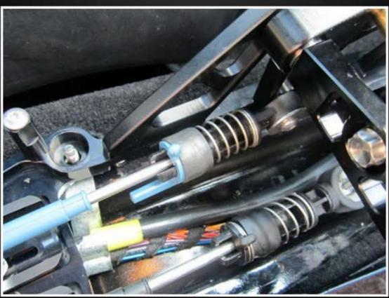
STEP 10: THERE WILL BE (4) 10MM NUTS HOLDING THE SHIFTER HOUSING IN. REMOVE THEM AND TAKE THE SHIFTER OUT OF THE CAR.
