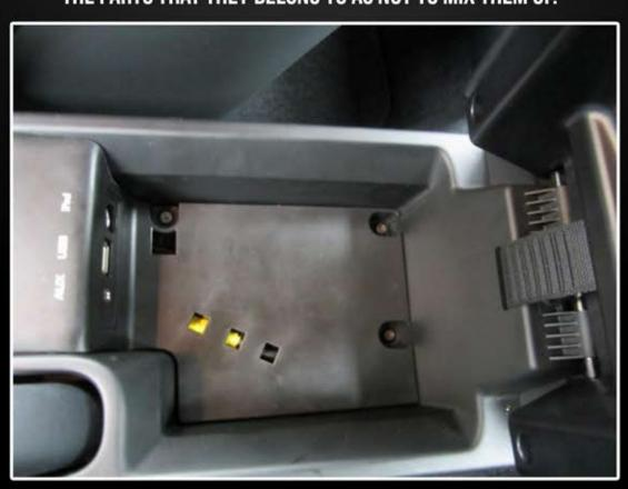
STEP 2: REMOVE THE COVER IN FRONT OF THE EMERGENCY BRAKE HANDLE BY PULLING UP ON THE FRONT FIRST AND REMOVE THE TORX SCREW.
