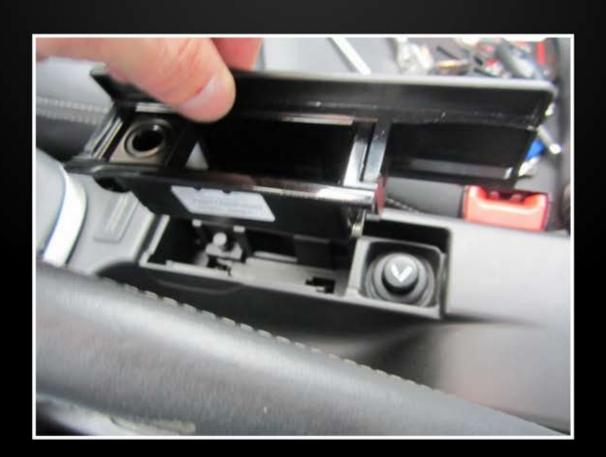
STEP 4: NOW YOU NEED TO REMOVE THE SHIFTER BOOT BY PULLING UP ON THE FRONT FIRST TO NOT BREAK THE TABS OFF. IT WILL JUST POP OUTOF THE TABS. THEN YOU HAVE TO TURN THE PLASTIC LOCK UNDER THE BOOT 90 DEGREES. PULL UP ON THE KNOB AND IT WILL SLIDE OFF.
