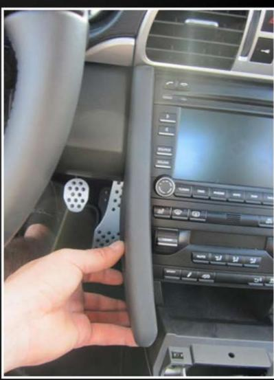
STEP 7: REMOVE THE T20 TORX SCREWS HOLDING THE VERY FRONT OF THE CONSOLE ON. NEXT REMOVE THE 2 T20 TORX SCREWS HOLDING THE STORAGE TRAY ON JUST BELOW THE RADIO. PULL THE STORAGE TRAY OUT BY PULLING IT STRAIGHT OUT. LAST REMOVE THE ONE T20 TORX SCREW UNDER THE STORAGE TRAY HOLDING THE CONSOLE IN.
