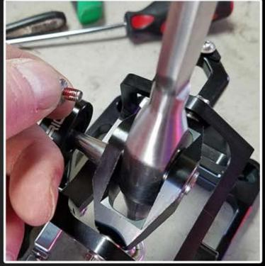
IF YOU ARE GOING TO RUN THE SHIFTER IN THE SHORTEST THROW POSITION (SHIFT LEVER IN TOP HOLE). YOU WILL NEED TO CUT AWAY A PIECE OF THE CARPET SO THE ROD END DOES NOT RUB ON THE CARPET. THIS WILL BE HIDDEN UNDER THE CONSOLE AND WILL NEVER BE SEEN. THE MAJORITY OF PEOPLE RUN THE SHIFTER IT IN THE MIDDLE POSITION.
