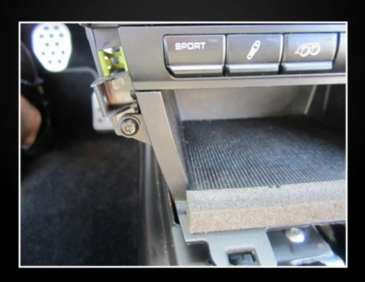
STEP 8: YOU ARE READY TO PULL THE CONSOLE OUT BUT FIRST LOCATE THE WIRE CONNECTOR ON THE INSIDE RIGHT FRONT OF THE CONSOLE ANDDISCONNECT IT. HAVE THE EMERGENCY BRAKE HANDLE PULLED UP. PULL THE CONSOLE UP AND OUT OF POSITION. YOU MAY HAVE TO REMOVE YOUR SEATS DEPENDING ON WHICH SEATS YOU HAVE. RECARO STYLE RACE SEATS THAT WRAP AROUND YOUR HEAD WILL NEED REMOVAL.
